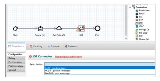
CoAP (Constrained Application Protocol) is an application layer protocol widely used in resource-constrained devices, such as wireless sensor nodes.
