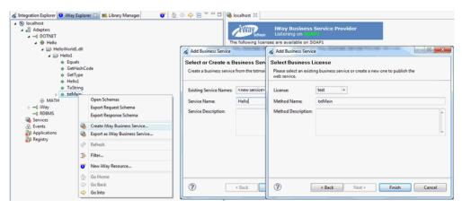
5. Display the newly created service (for example, *Hello*), by right-clicking the Services node and selecting *Connect* from the menu list if the Services node is not connected, or *Refresh* if the Services node has already been connected.
