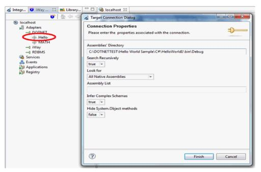
3. Export a request schema with a method (for example, *txtMain*) to an integration project, as shown in the following image.
